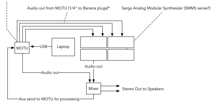
\*floating point value from Max is converted to control voltage (CV) used for modulating various analog synth parameters (frequency, amplitude, mod depth, sequence clock rate)
